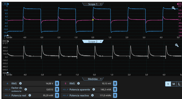
Figura 28: Stimulator working in VC mode on body tissues.
