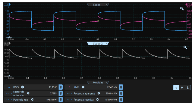
Figura 22: Application on body tissues with alternating quadrangular 4 KHz 12 Vp. Rubber electrodes with damp cloth.
